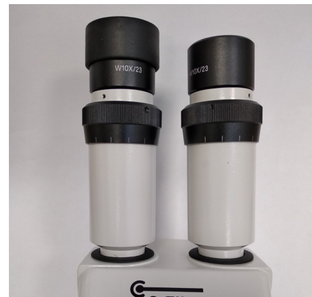
Figure 29 - Dioptré with and without the eyecup
