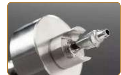
Usinage de piliers en titane Milling of titanium abutments Fresatura di abutment in titanio
