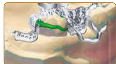
Crochet personnalisé Freeform design of the clasps Ganci personalizzati
